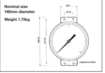
For Type 93 all other dimensions are as for Type 91 above except that the panel mounting bezel is replaced by a plain bezel.
