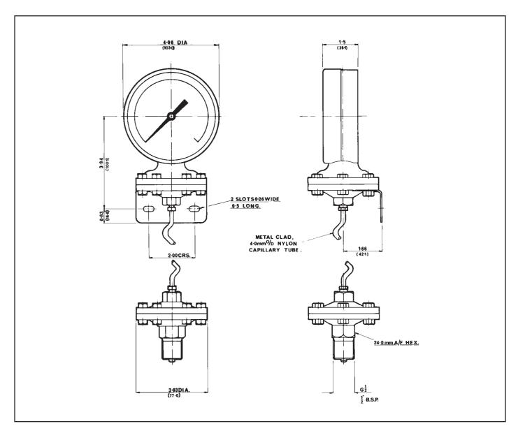
Bailey & Mackey diaphragm pressure gauges in ranges 0-1 bar and above can be fitted with transmitters for distant reading. In this way indication can be provided at a panel some distance away from the tapping point or, where severe vibration is present, the gauge can be mounted on a wall away from the vibration.
