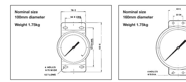
For Type 97 all other dimensions are as for Type 95 above except that the panel mounting bezel is replaced by a plain bezel.
