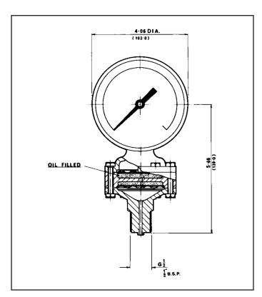
In many applications where diaphragm gauges are used it is not possible to protect the mechanism against the effect of pulsating pressures by means of a snubber involving a small orifice in the line to the gauge. This particularly applies where the application is on suspended solids or there is a hygiene requirement. The Bailey & Mackey solution to the problem is integral hydraulic throttling.
