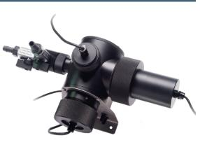
The TurbiTechw<sup>2</sup> LR Sensor has been specifically designed to monitor final treated, potable and filter water. The sensor is extremely sensitive and is capable of discriminating changes in Turbidity of less than 0.1 FTU. The 90° light scatter monitoring technique makes the sensor sensitive to a wide range of particle sizes, from colloidal material throughto larger particles, raw water and the large mineral particles sometimes found in distribution samples.
