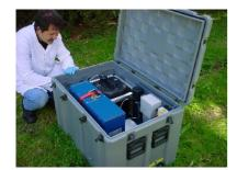
This site evaluation package allows the user to quickly assess problems that a site is encountering by monitoring 24 hours per day and at weekends. Data from site evaluations has already allowed water company's to identify site process problems and to track down illegal dumping of chemicals into the water course by an unscrupulous manufacturer.
