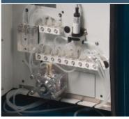
The MicroMac C is designed to operate in an industrial or treatment works environment with minimal routine intervention and uses wherever possible industry standard chemistry methods. The robust nature of the MicroMac C with its separate electronic and chemistry compartments the latter including reagent storage provides a highly reliable on-line analyser.
